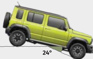
RAMP BREAKOVER ANGLE
